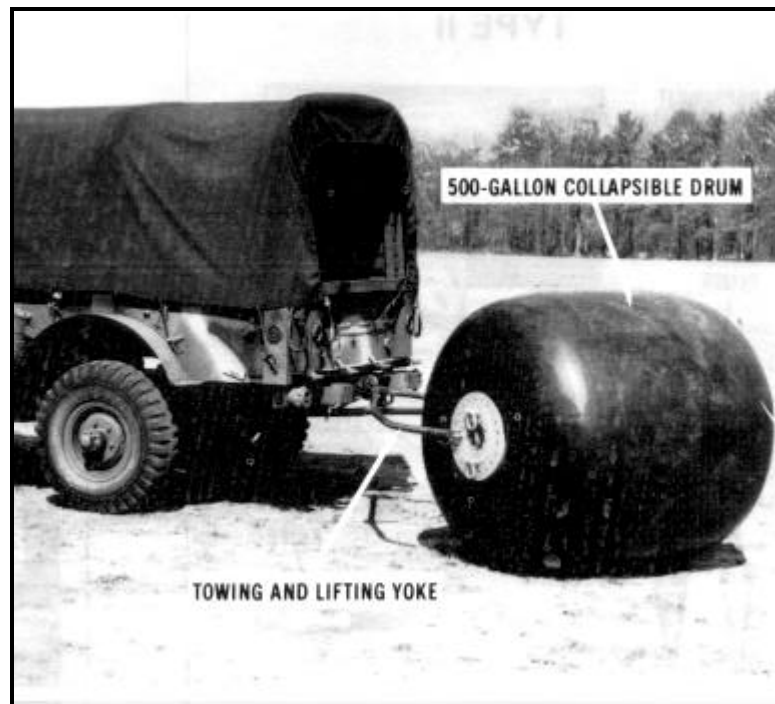
Figure 22-12. Filled 500-gallon drum being towed by cargo vehicle
