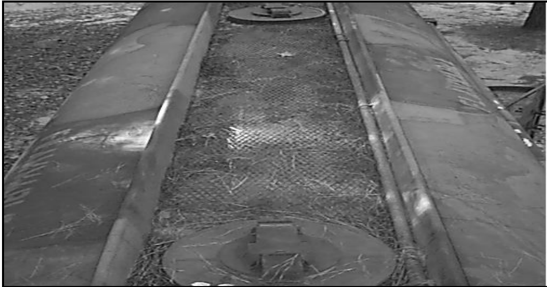
Figure 24-12. Manhole and filler covers and walkway of the M131A5C and M131A5 tank
