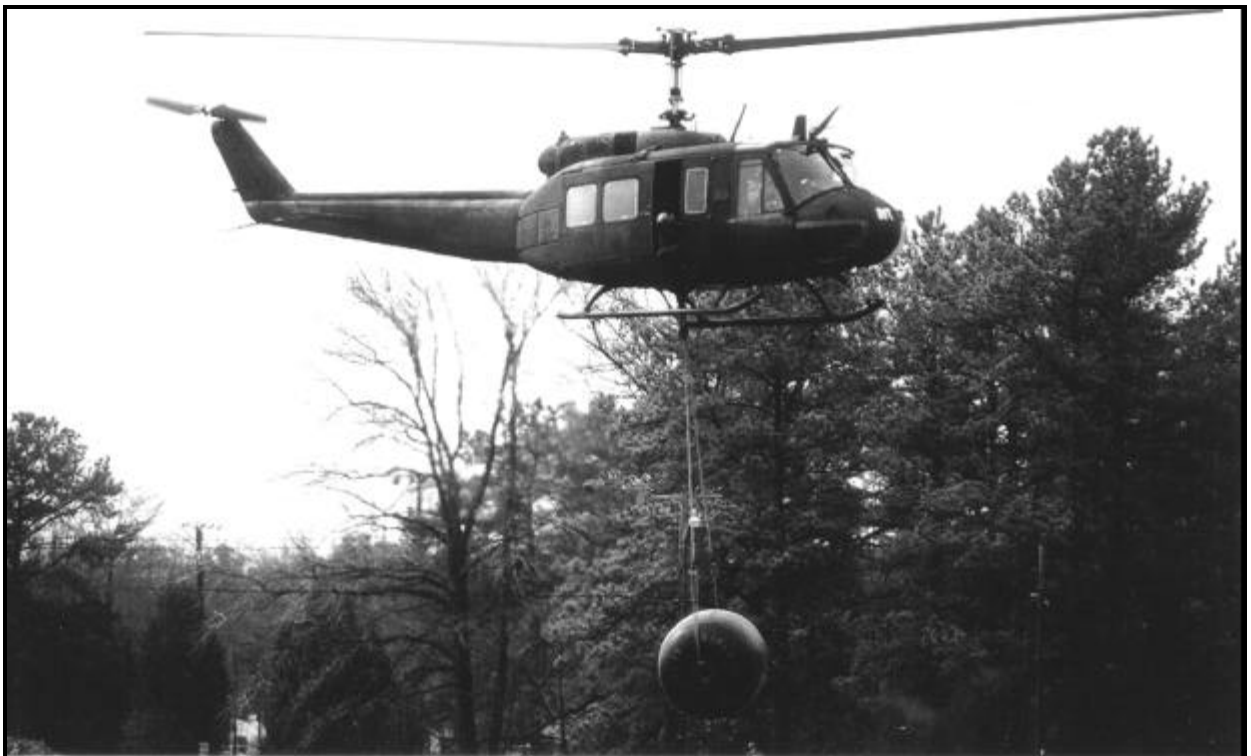
Figure 22-14. Helicopter carrying filled 500-gallon drums
